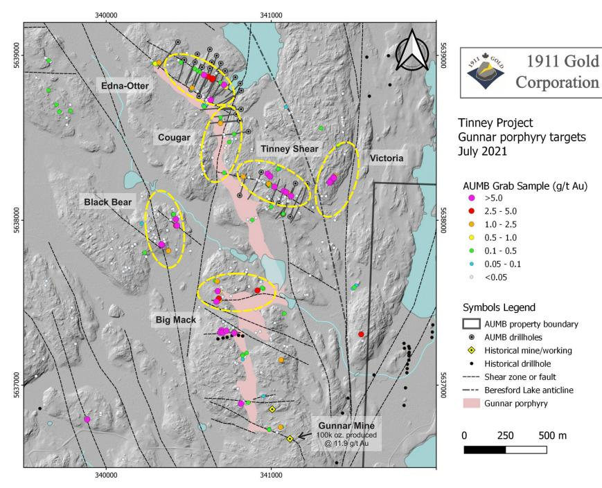
Figure 2: Tinney project area, with gold showings, previous drilling and interpreted structure over LiDAR base.
